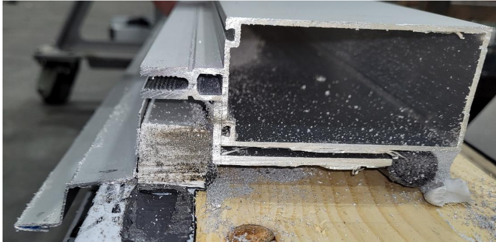
Photo No. 3 Sill assembly
