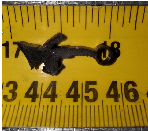
Photo No. 18 Glazing Gasket
