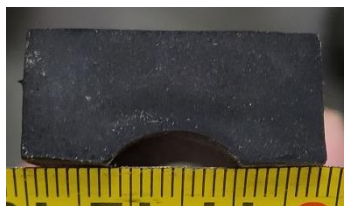
Photo No. 14 Setting block profile
