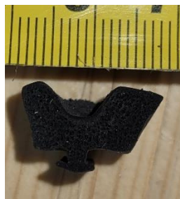
Photo No. 8 Interior glazing gasket
